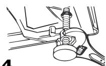
If washer is not level, screw the front legs up or down to adjust. Make final check with
